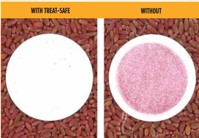
Dust-off filter paper testing demonstrates a vast reduction of dust when Treat-Safe™ is applied with seed treatments.
